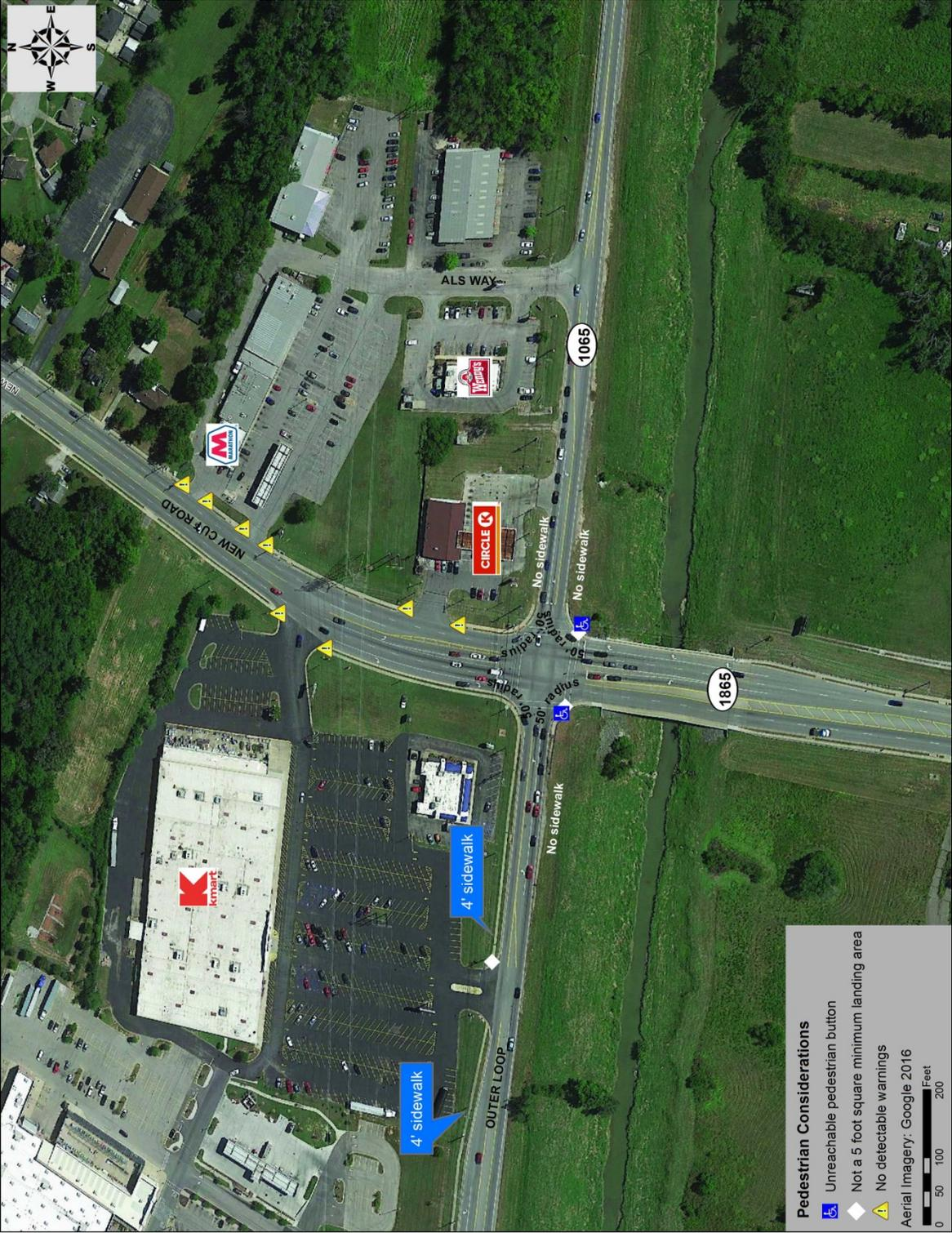
Figure 3.22: Outer Loop/New Cut Road Pedestrian Accommodations and Signal Analysis
